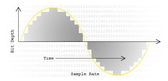
Bit Depth refers to the number of bits you have to capture audio. The easiest way to envision this is as a series of levels, that audio energy can be sliced at any given moment in time. With 16 bit audio, there are 65,536 possible levels. With every bit of greater resolution, the number of levels double. By the time we get to 24 bit, we actually have 16,777,216 levels. Remember we are talking about a slice of audio frozen in a single moment of time.
